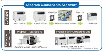
Convert manual insertion process to SMT inline process Reduce processes / dip solder investment
