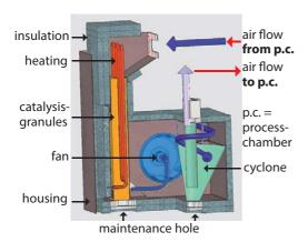
The catalysis - process gas cleaning can be installed into the SMT reflow soldering system XS and in all reflow soldering systems from the Quattro Peak series. Depending on the system size, this may be up to 4 catalysis (up to 5 at vacuum soldering systems).
